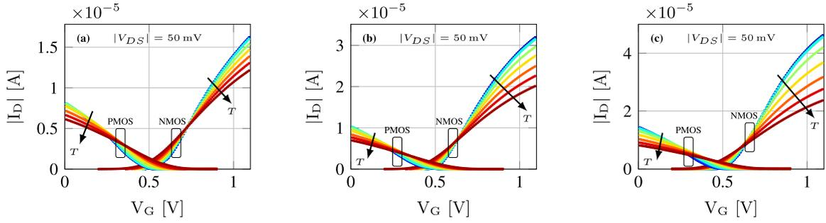
**FIGURE 6.**  $I_D - V_G$  curves as function of temperature for: a) NMOS/PMOS  $W/L = 120\text{n}/40\text{n}$ ; b) NMOS/PMOS  $W/L = 360\text{n}/120\text{n}$  and c) NMOS/PMOS  $W/L = 1.2\mu/400\text{n}$ .  $T = 4.2, 10, 40, 50, 100, 150, \dots, 300\text{ K}$ .  $V_S = 0\text{ V}$  and  $V_D = 1.1\text{ V}$  for NMOS and PMOS, respectively.
