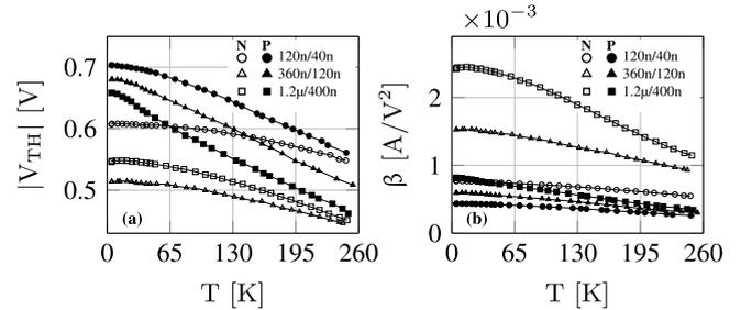
**FIGURE 7.** Threshold voltage (a) and current factor (b) as a function of temperature for NMOS and PMOS devices with different geometries.
