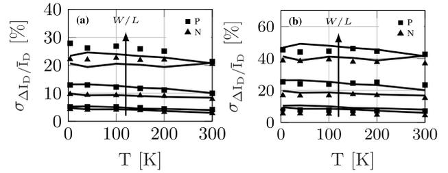
**FIGURE 11. Drain-current mismatch as a function of temperature at a fixed  $G_m/I_D$  in saturation ( $V_{DS} = 1.1\text{ V}$ ). a)  $G_m/I_D = 5\text{ V}^{-1}$ ; b)  $G_m/I_D = 10\text{ V}^{-1}$ . Marks: measured data, lines: simplified Croon model as in Eq. (2). Arrow points in direction of decreasing W/L: 1.2  $\mu\text{m}/40\text{n}$ , 360n/120n and 120n/40n.**
