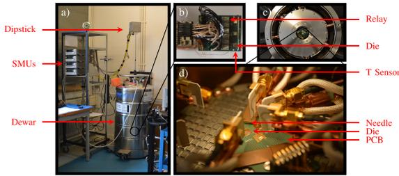
**FIGURE 4. Measurement setup. a): dipstick; b) detail of PCB on the dipstick. The temperature sensor (Cernox RTD) is located on the opposite side of PCB. Relays used for die selection; c) cryogenic probestation; d) detail of the PCB in the cryogenic probestation.**
