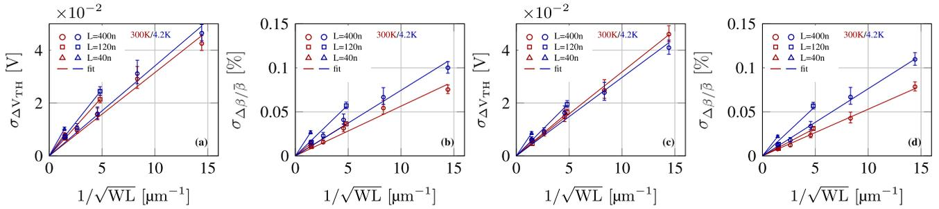
**FIGURE 8.** Pelgrom plots for  $V_{TH}$  and  $\beta$  with length dependency indicated by separate fitting for each length at RT (red) and LHT (blue). a), b) NMOS; c), d) PMOS. Error bars indicate 95% statistical confidence intervals.
