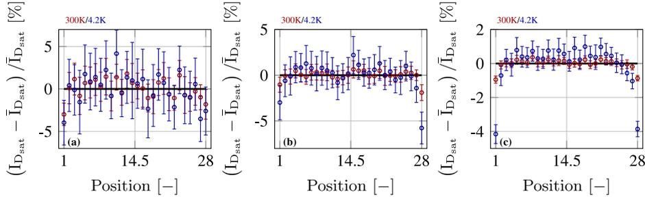
**FIGURE 13.** Relative  $I_{D_{sat}}$  ( $I_D|_{V_{DS}=V_{GS}=1.1\text{ V}}$ ) values as a function of device position for PMOS devices at RT (red) and LHT (blue): a)  $W/L = 120\text{n}/40\text{n}$ ; b)  $W/L = 360\text{n}/120\text{n}$  and c)  $W/L = 1.2\mu/400\text{n}$ . Zero deviation emphasized by the black lines and error bars indicate 95% confidence intervals.
