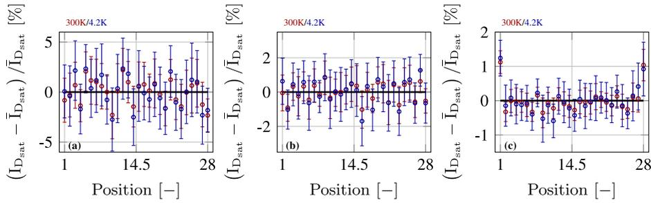
**FIGURE 12.** Relative  $I_{D_{sat}}$  ( $I_D|_{V_{DS}=V_{GS}=1.1\text{ V}}$ ) values as a function of device position for NMOS devices at RT (red) and LHT (blue): a)  $W/L = 120\text{n}/40\text{n}$ ; b)  $W/L = 360\text{n}/120\text{n}$  and c)  $W/L = 1.2\mu/400\text{n}$ . Zero deviation emphasized by the black lines and error bars indicate 95% confidence intervals.
