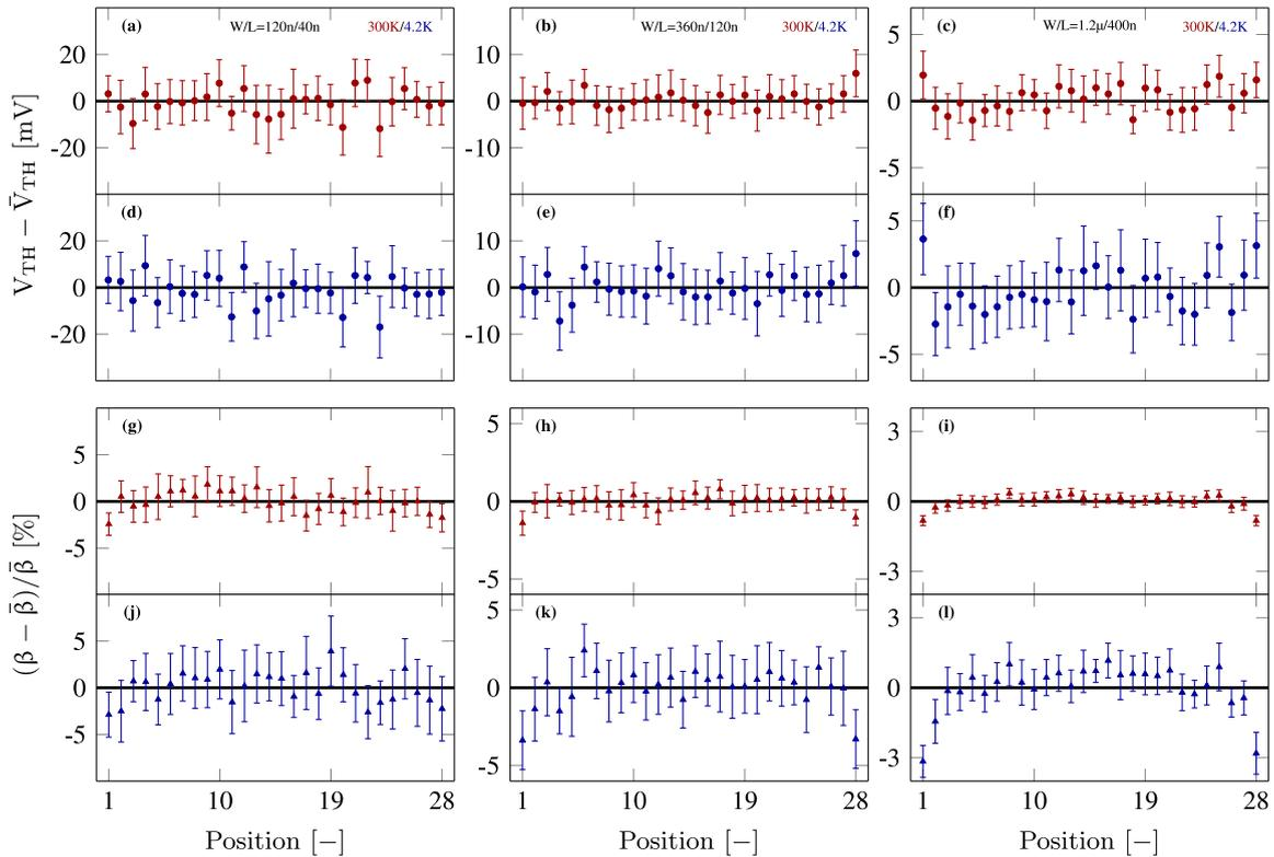
**FIGURE 15.** Normalised  $V_{TH}$  (circle) and  $\beta$  (triangle) as a function of device position for PMOS devices at RT (red) and LHT (blue). First column:  $W/L = 120n/40n$ ; second column:  $W/L = 360n/120n$ ; third column:  $W/L = 1.2\mu/400n$ . Error bars indicate 95% confidence intervals.
