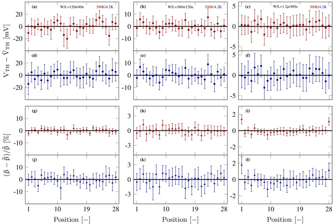
**FIGURE 14.** Normalised  $V_{TH}$  (circle) and  $\beta$  (triangle) as a function of device position for NMOS devices at RT (red) and LHT (blue). First column:  $W/L = 120n/40n$ ; second column:  $W/L = 360n/120n$ ; third column:  $W/L = 1.2\mu/400n$ . Error bars indicate 95% confidence intervals.
