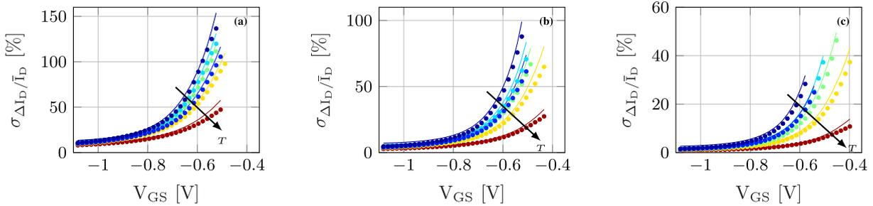
**FIGURE 10.** Drain-current mismatch for PMOS devices as a function of temperature ( $|V_{DS}| = 50$  mV).  $T = 4.2, 40, 100, 150, 200$  and  $300$  K. a)  $W/L = 120n/40n$ ; b)  $W/L = 360n/120n$ ; c)  $W/L = 1.2\mu/400n$ . Dots: measured data; lines: simplified Croon model as in Eq. (2).
