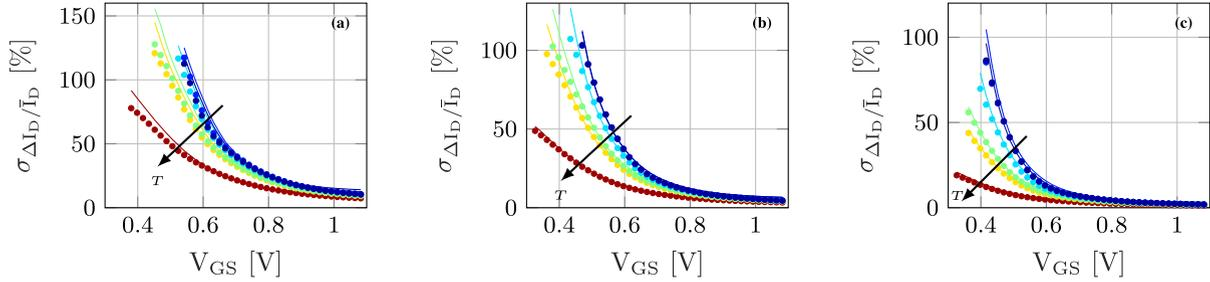
**FIGURE 9.** Drain-current mismatch for NMOS devices as a function of temperature ( $V_{DS} = 50$  mV).  $T = 4.2, 40, 100, 150, 200$  and  $300$  K. a)  $W/L = 120n/40n$ ; b)  $W/L = 360n/120n$ ; c)  $W/L = 1.2\mu/400n$ . Dots: measured data; lines: simplified Croon model as in Eq. (2).
