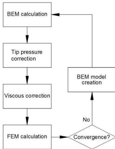
Figure 3: Flowchart of the coupling scheme.
