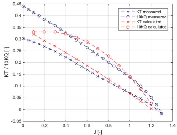
**Figure 5: Calculated and measured open-water diagram.**
