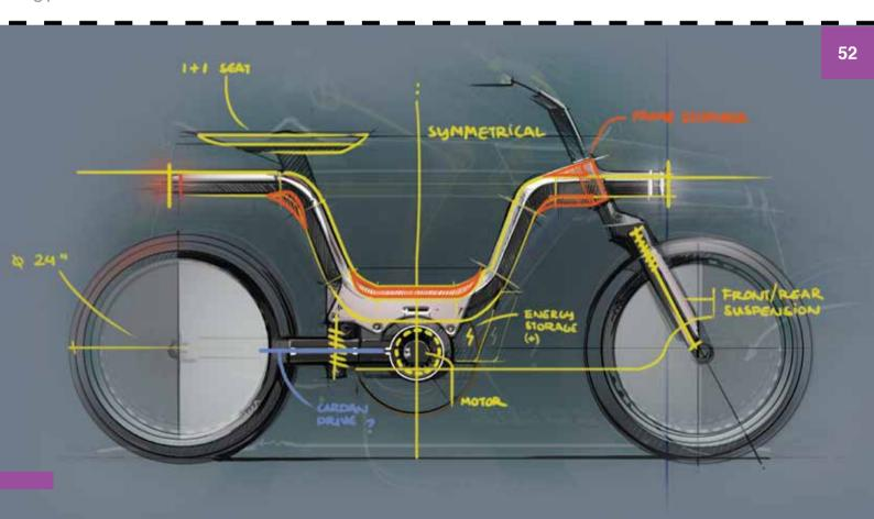
drive-shaft also proves to be a cleaner solution when compared to a chain or belt, since the system is closed.
