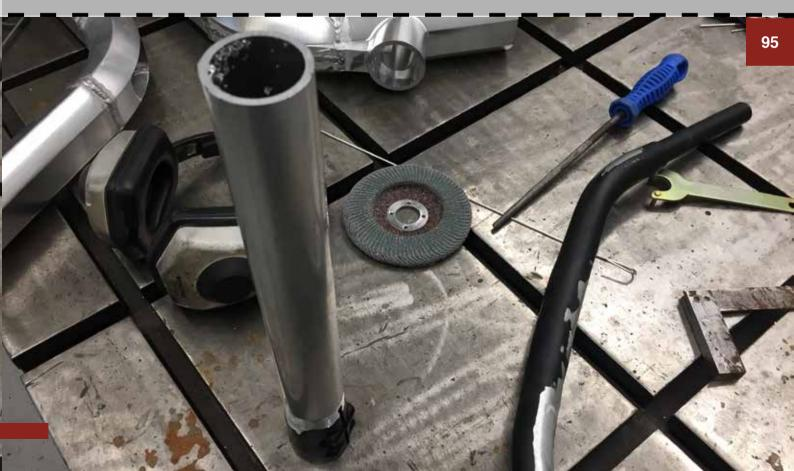
Finding an appropriate suspension 24 inch front fork proves to be very difficult due to the Covid-19 induced lock-down. For this reason, a set of temporary adapter units are turned on a lathe in order to install a front fork as currently used in the X3 model 98. This allows the frame to roll and be tested without having a suspension fork just yet 99. With this temporary setup it was concluded that no parts failed under load!
