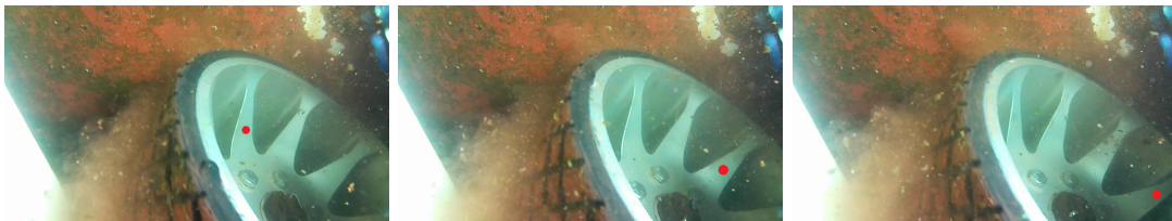
Figure 2-1: Images captured of wheel slipping in longitudinal direction. The red dots mark the same spoke in a time span of 1 second. The images show that although the wheel is rotating, the robot remains stationary.
