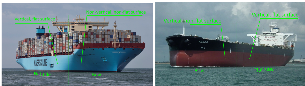
Figure 6-2: Images of oceanic trade vessels, displaying the ship hull shape. Left: Mc-Kinney Møller, container transport vessel [100]. Right: Teseo, crude oil tanker [101].
