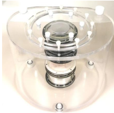
Figure 17 PET phantom box assembly of the first prototype in the NEMA body PET box as designed in (V.7)
