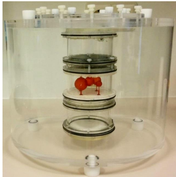
Figure 59 PET phantom assembly of all the segments including the one containing the spherical inserts before filling (center).
