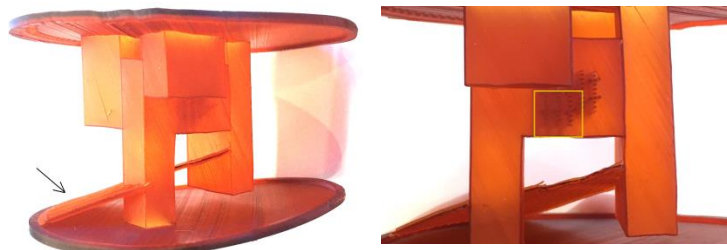
Figure 36 SLA print of the phantom cubical insert (V.3.4)
