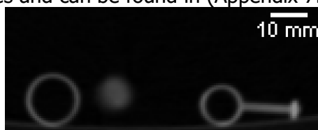
Figure 43 Transversal CT image view of the spherical V.3 inserts in air Transversal view of the sphere of 17mm inside diameter (left), blurry top view of the 22mm diameter sphere (middle), side view of the smallest sphere (10mm diameter).
