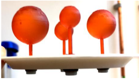
Figure 55 Assembly of the spherical inserts with their holding plate, leaks appear at the bottom of the plat where each sphere is closed by a M3 screw
