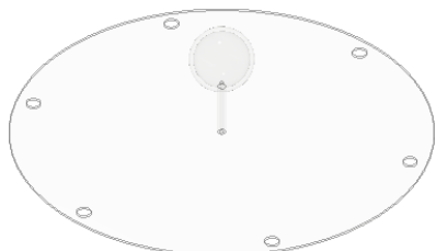
Figure 20 Phantom spherical insert design (V.1)
