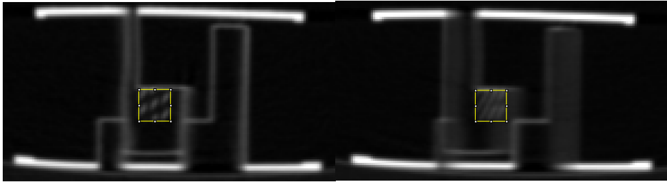
Figure 54 CT acquisition of semi filled cubical insert
