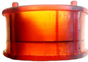
Figure 9 Lateral view of the SLA printing of a miniaturized version 0 of the phantom box (V.0) Even if a thin wall thickness (1mm) the printed material is too opaque for the phantom imaging segments.
