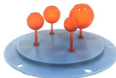
Figure 25 Phantom spherical FDM printed insert (V.5) with the four SLA printed spheres attached to one of its side
