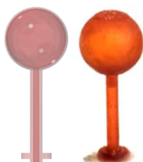
Figure 19 Photopolymer R05 as designed (left) and printed (right) (extracted view from Inventor®)
