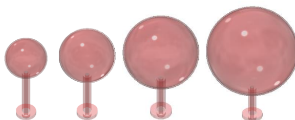
Figure 22 Phantom spherical insert design (V.3.2): spheres of 10, 13, 17, and 22mm ID
