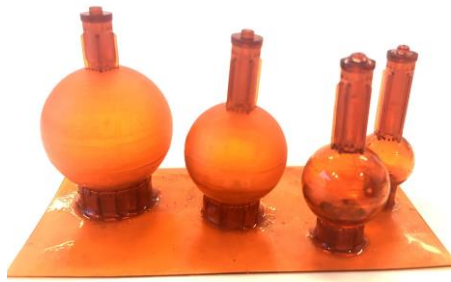
Figure 23 Phantom spherical insert design (V.3.2) SLA 3D printed with support
