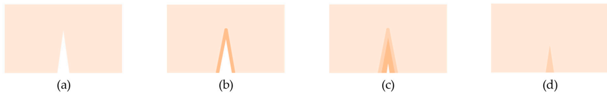
Figure 1. The basic principle of crack healing in asphalt pavement: (a) a crack generated in asphalt mastic; (b) the ‘mobile phase’ induced at the crack face; (c) closure of the crack by the ‘mobile phase’ and (d) immobilisation after healing (Hager et al., 2010).
