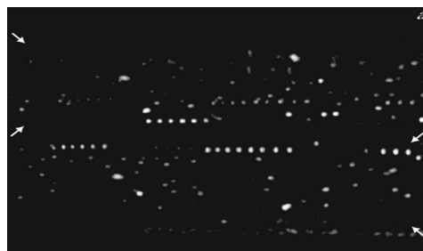
Figure 2.12: Image of Trains of Particles. Figure is reproduced from Matas et al. [21]
