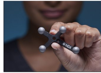
Figure 1: NDI optical marker with 4 reflective spheres used in medical practices [5]
