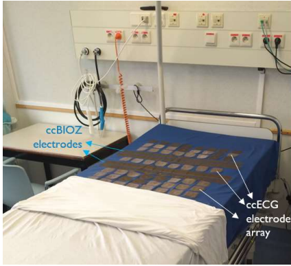
Figure 1. Mattress with ccECG and ccBioz sensors installed at the sleep laboratory. Cover partially removed for the picture (bed fully covered when collecting data).
