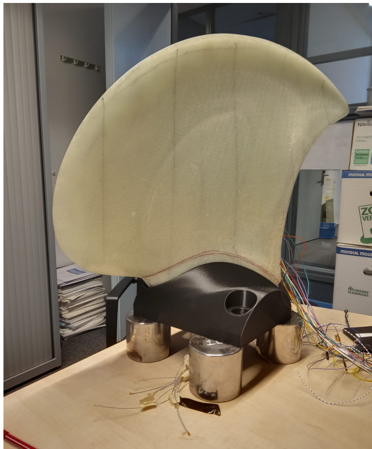
Figure 2.10: Doubly curved propeller blade made of GFRP
