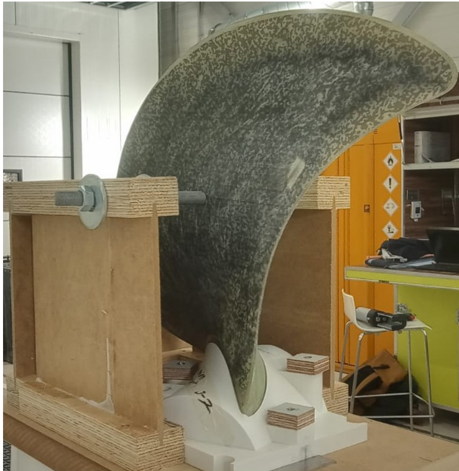
Figure 6.21: Actual blade: fabrication of the hub-blade interface
