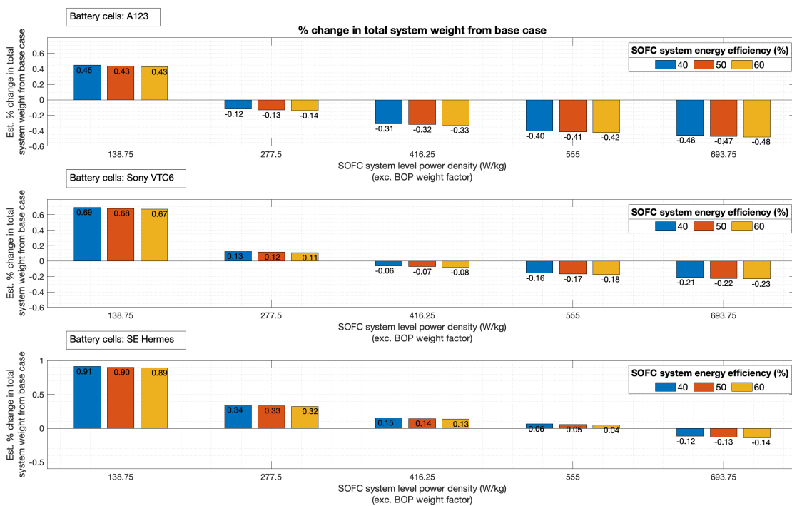
Figure 5.6: Mass comparison against base case for E65-FC SOFC-BT(Variable)-CFCCruise
