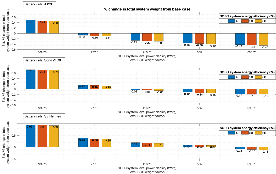
Figure B.11: Weight comparison against base case for E110-FC SOFC-PD(Variable)-BT(Variable)-CFCCruise
