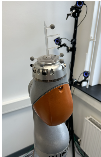
Figure 2.4: 3D-printed end-effector with iterated design improvements and threaded attachment points for 12 mm OptiTrack markers.
