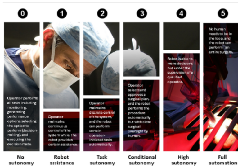
Figure A.1: Different levels of autonomy in robotic surgery as presented by Yang et al. [4], based on the SAE levels of driving automation.
