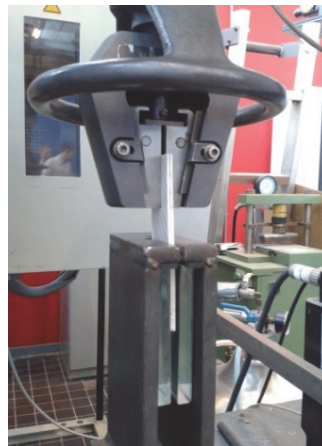
Fig. 35, 36 Pull out test customized configuration
