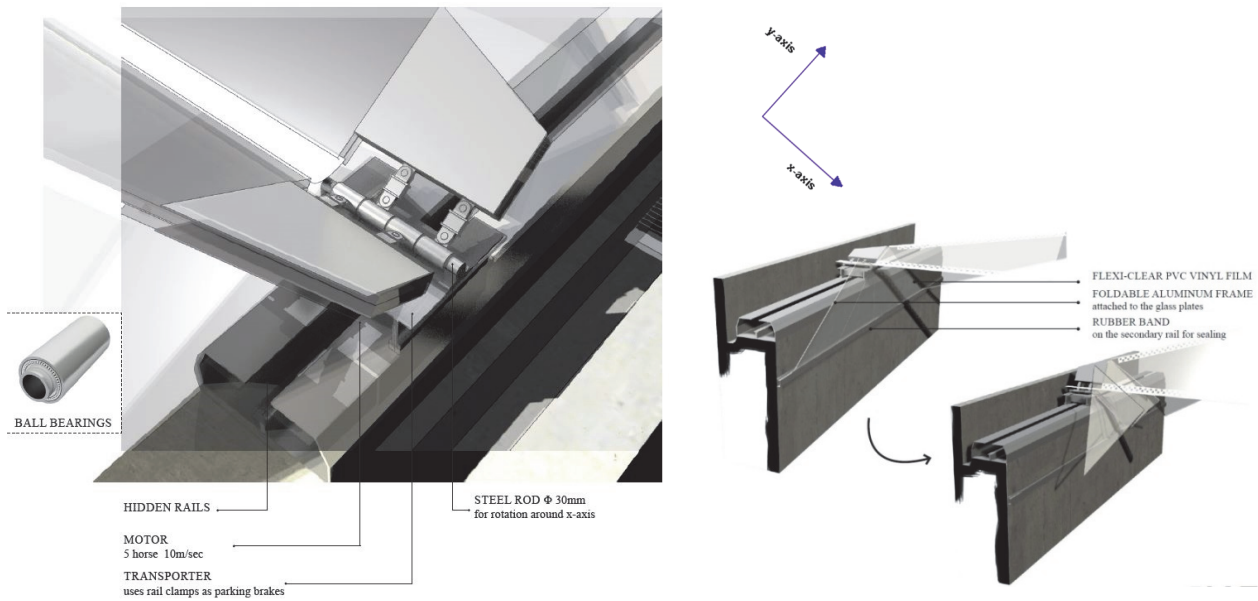
Fig. 15,16 Deployment on parallel rails mechanical system detail and waterproofing detail on the structure to wall connection and the railing system, on the deployed and un-deployed state.
