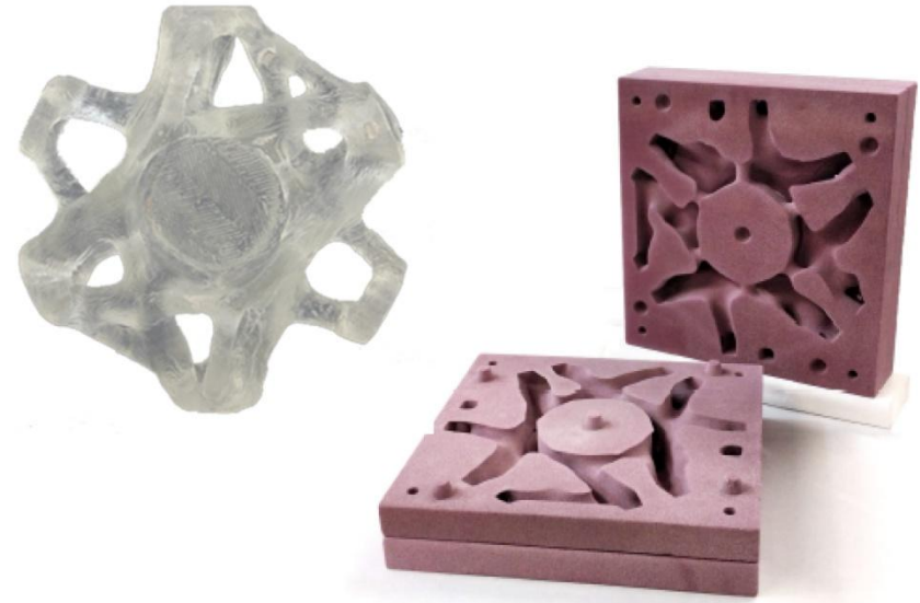
Damen, W. (2019). Topologically Optimised Cast Glass Grid Shell Nodes
