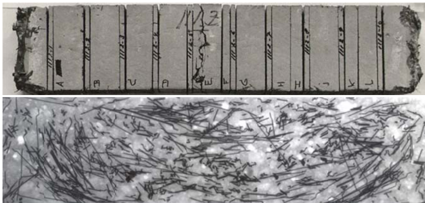
Fig. 6. (bottom) X-ray radiograph of a “vertical slice” (totaling 10 in this case) of a test-loaded (and cracked) SFRC specimen of 70x200x1000 mm (top). Compaction by gravitation was in vertical direction. Analysis is by orthogonal line grids.
