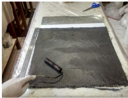
28 Fig. 1 Carbon fiber lamination process 29 30 31 32
