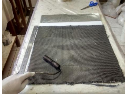
Fig. 1 Carbon fiber lamination process
