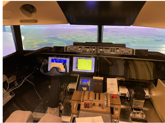
Figure 4. The simulator's flight deck emulating the Piper Seneca III with Garmin avionics.
