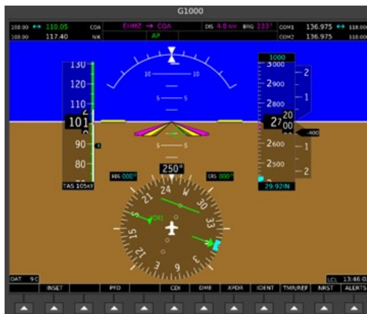
Figure 6.2: PFD of G1000 50 seconds into the Engine Out scenario. No roll angle visible, FPV indicates remaining sideslip
