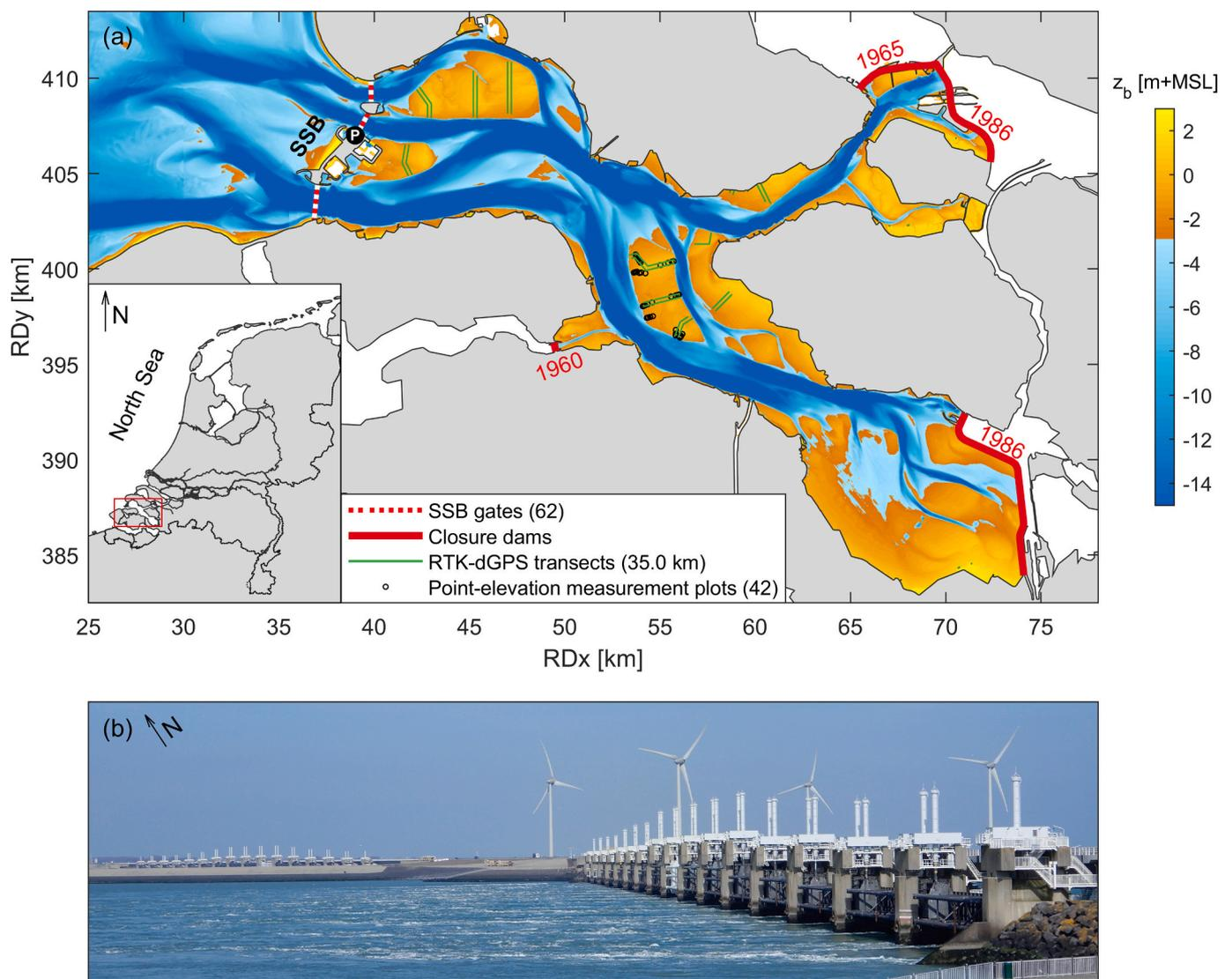
**Fig. 1.** Bathymetry of the Eastern Scheldt of 2019 (a) with the storm surge barrier (SSB), closure dams (years of closure indicated in red) and the location of the RTK-dGPS transects and point-elevation measurements. The maximum depth of the channels exceeds the color scale, see Fig. 3a for the full elevation distribution. A photo of the SSB gates is provided in (b), taken on 23 March 2017 at location P in (a) looking at the NNE.
