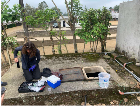
FIGURE 8: Chlorine testing of cistern water
