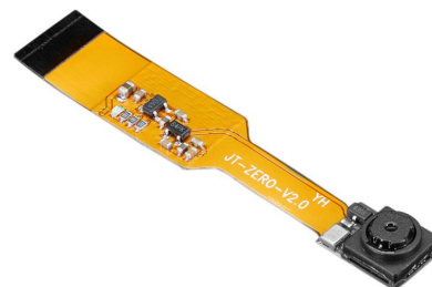
(b) Camera module Zero Spy Camera
