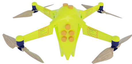
Figure 7.13: Drone with fluorescent yellow livery and reflective stickers on the arms
