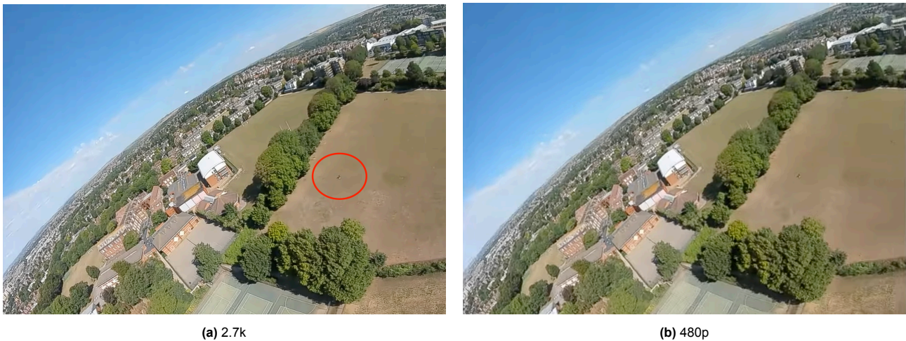
Figure 12.2: Comparison of the same drone shot with different video quality where the spot in the middle of the red circle in 12.2a is a person for reference purposes at an altitude of 50 meters approximately
