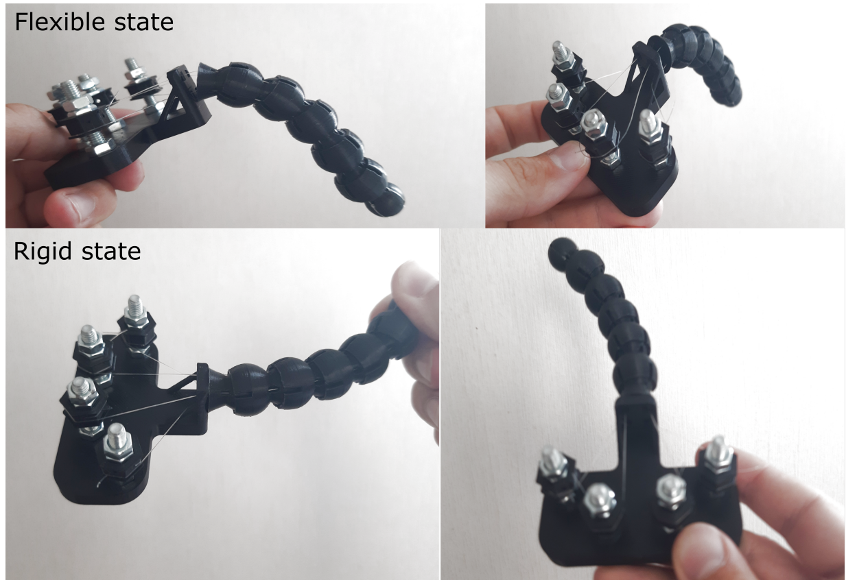
Figure 25: First concept of the segment jamming mechanism in flexible and stiff state. The ball and socket joints can be fixed to each other by tightening the screws on the frame which applies tension to the wires.
