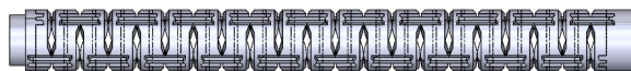
Figure 9: Improved Sheath design that consists of 20 joints connected by a compliant flexure.
