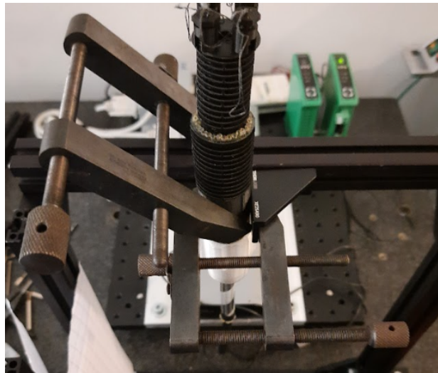
Figure 23: Fixation of the prototype with two claps around the mechanism.
