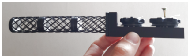
Figure 7: Phase change mechanism consisting of multiple steering segments (black braided structures) and steered by two wheels.
