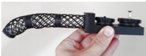
Figure 8: Phase change mechanism in its curved configuration.
