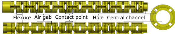
Figure 12: Schematic overview of the steerable segment. The flexure connects two segments together which have a single point of contact over which it can bend. There are four steering channels and a central channel.
