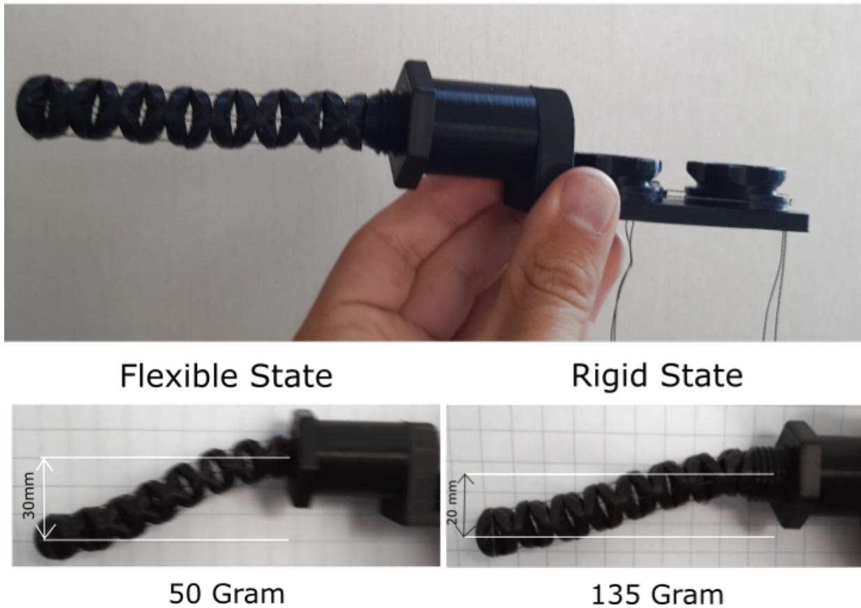
Figure 27: Third concept of segment jamming mechanism. The mechanism is steered by two wheels and stiffened by a screw mechanism. The joints used in this concept are the rolling friction joints. The bottom shows a stiffness test. On the left the deflection of the mechanism in flexible state with a load of 50 gram. On the right the deflection of the mechanism in stiff state with a load of 135 gram.
