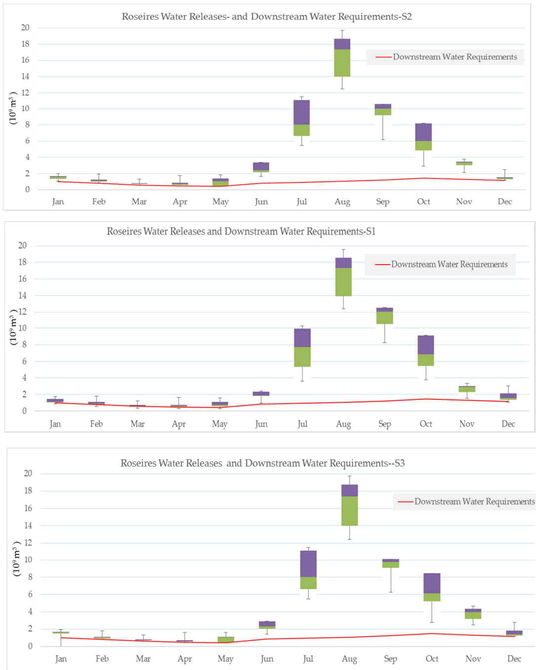
Figure 6.6 Releases from optimization scenarios and monthly downstream water requirements (including Gezira and Managil irrigation demand), averaged for the period of 1993–2012
