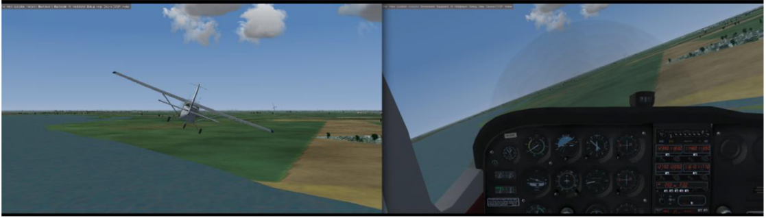
Figure 1. A situation of a bank angle from an external perspective, seen from behind the aircraft (left), and as seen from the cockpit (right).
