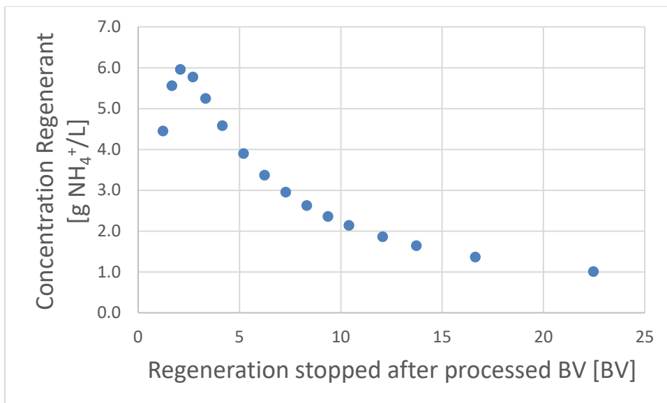
Figure 21: IEX Laboratory Set-Up: Regeneration with 100 g NaCl/L: Calculation of the maximum \text{NH}_4^+ concentration of the Regnerant after processed BV. Maximum concentration after 2.1 BV (6.0 g \text{NH}_4^+ /L)
