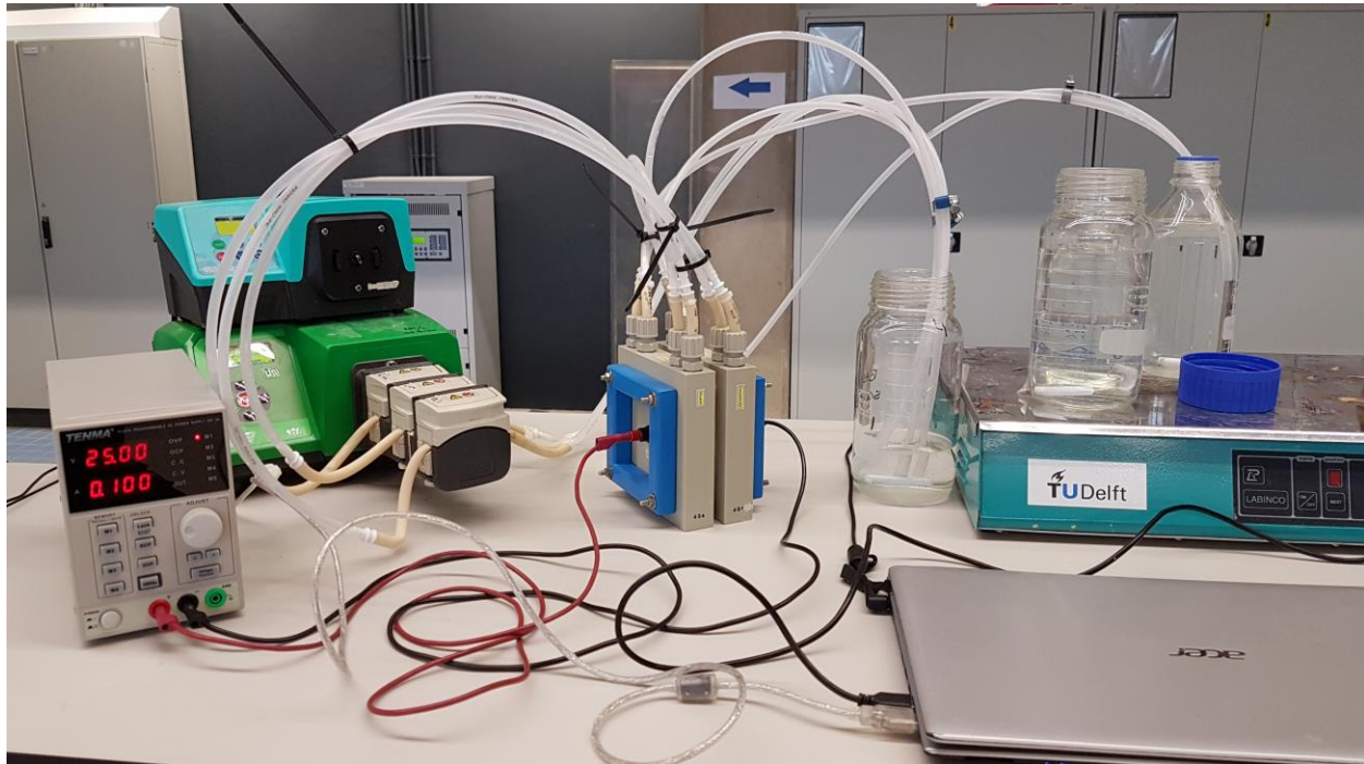
Figure 13: Photo of ED Laboratory Set-Up; Concentrate, diluate and electrolyte were recirculated in the three reservoirs (right), pumped by (green) pumps. The current was provided by Tenma DC Power Supply (left), a laptop was used to log measurements.
