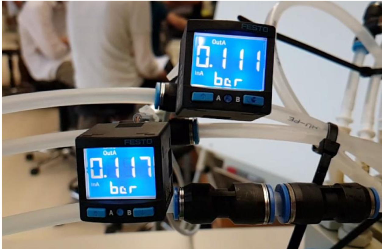
Figure 41: Photo of Pressure Sensors: Calculating Power [W] of the Pumps used in ED Laboratory Experiments.
