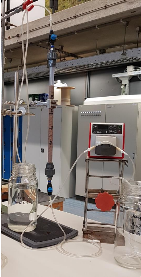
Figure 11: Photo of IEX Laboratory Set-Up; Regenerant (right reservoir) was pumped up through the IEX bed and collected in clean reservoir (left).
