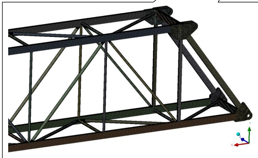
Figure 147: Applied mesh and typical detail for clarity
