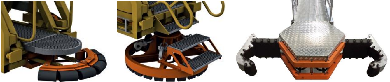
Figure 11: Different landing mechanisms for the gangway
