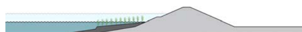
Figure 1: Coastal defence system of a hard engineered infrastructural measure (dike) with an adjacent dynamic ecological zone (a salt-marsh zone) [source: 25].
