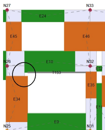
Figure 6.20: Missing connection in the mesh.
