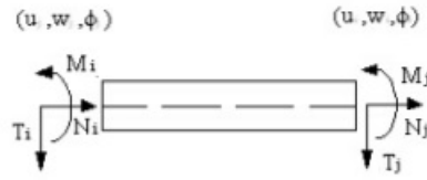
Figure 3.14: Macro-element 3Muri. Source: S.T.A. DATA srl
