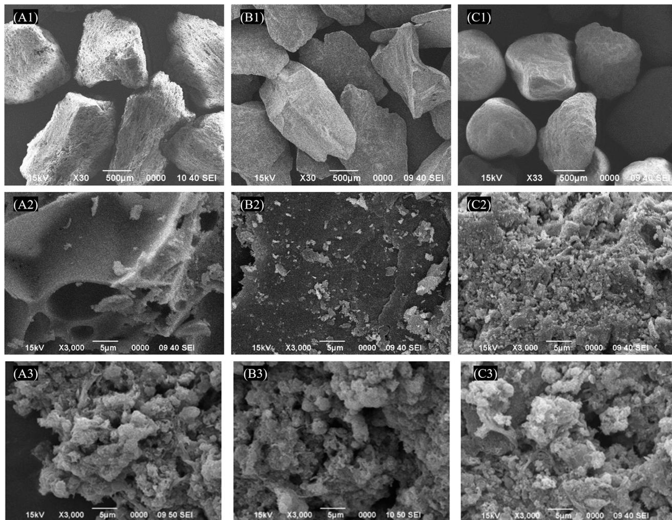
Fig. 6 Scanning electron microscopy (SEM) images with a magnification of 30 $\times$  and 3000 $\times$  of (A) pumice stone (B) anthracite, and (C) silica sand.
