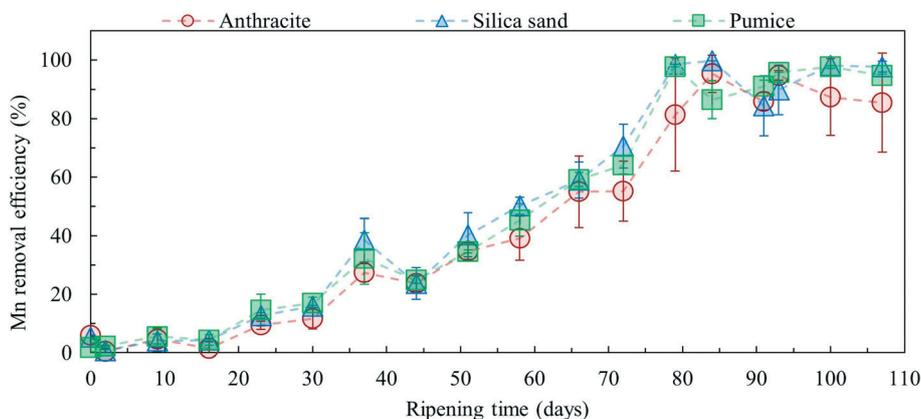
Fig. 2  $\text{Mn}^{2+}$  removal efficiencies in anthracite, silica sand, and pumice stone columns (error bars represent standard deviations).
