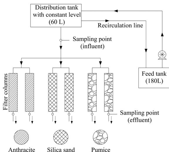
**Fig. 1** Configuration of the experimental unit.
