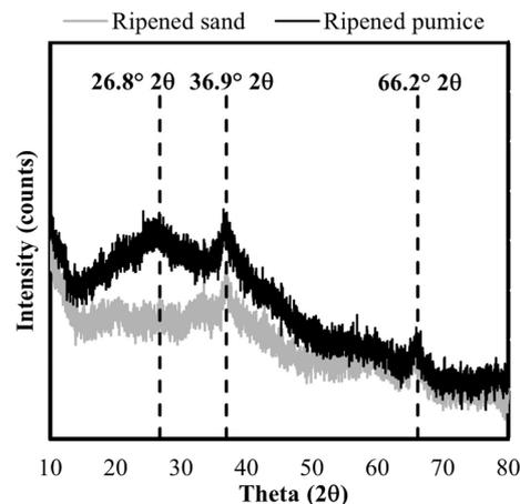
Fig. 5 XRD patterns of MnO<sub>x</sub> deposits obtained on the surface of ripened silica sand and ripened pumice.
