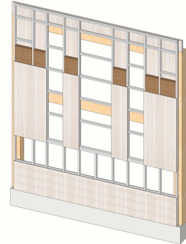
osb panel + thermal insulation material
