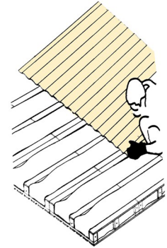
3. The corrugated aluminum sheeting is placed on top of the pallet structure.
