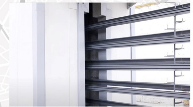
4. Heat aluminum profiles in the curing oven
