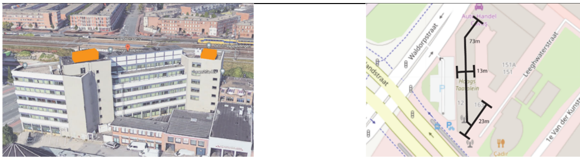
Figure 102: Picture of lift shafts and plot of Calandstraat 12 with rough measurements on an edited map from Open Street Map (N.D.) (Google Earth, N.D.)
