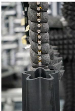
(a) Lobed nozzle with peak orientated to the linear array.
