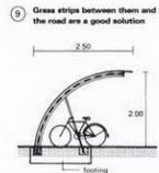
⑬ Weather protection roof - curved roof
