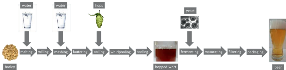
Figure 2: Schematic representation of the beer brewing process. Carbohydrates from cereal grains are extracted through germination (malting), mixed with water and broken down into fermentable sugars (mashing). After separation from spent grains, hops are added to the resulting sweet broth (wort). Wort sugars are converted by brewing yeast into CO 2 and ethanol and after conditioning, the final product, beer, is ready.
