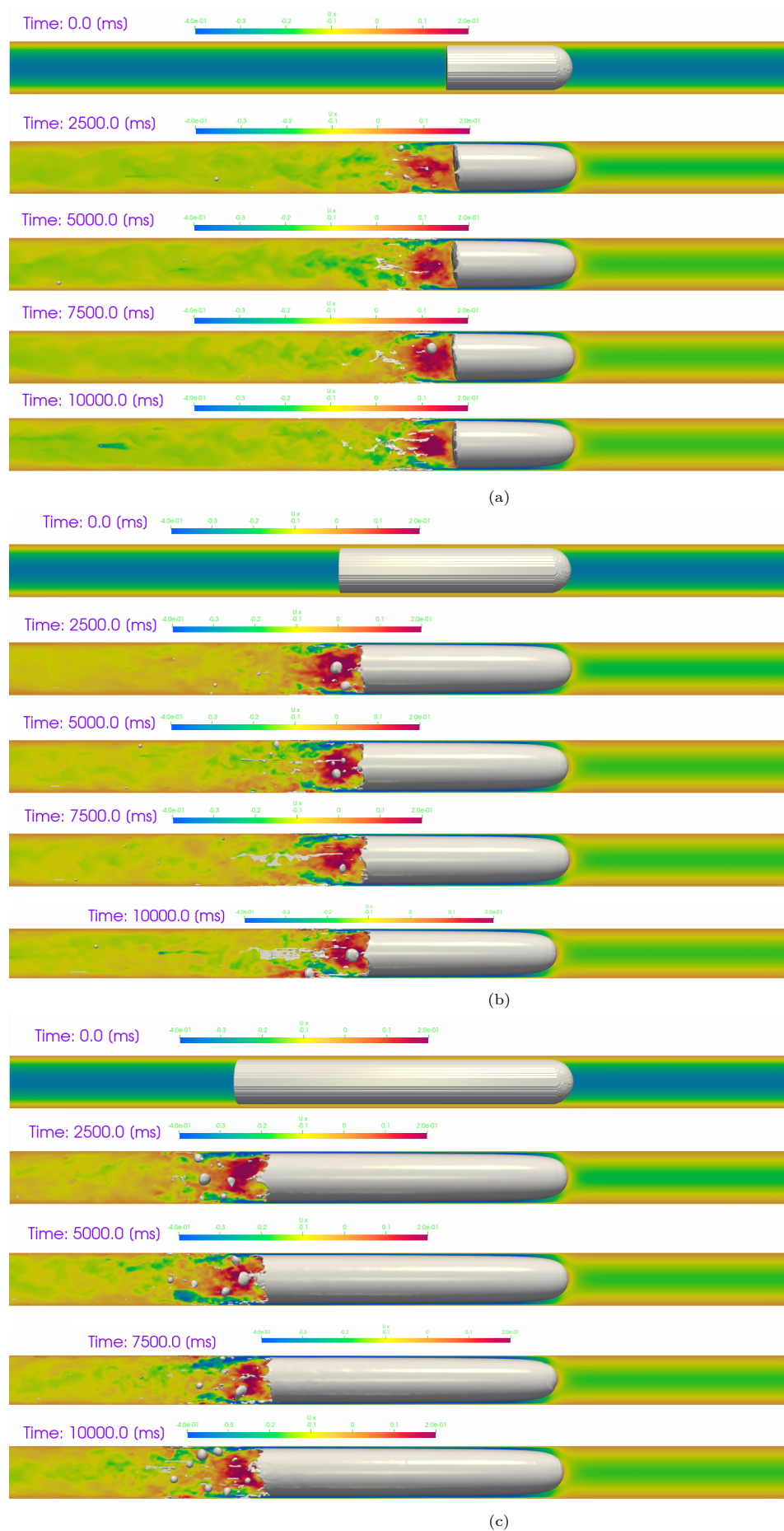
Figure 5.2: Time evolution of liquid streamwise velocity and bubble behaviour for simulations of laminar counter-current Taylor bubble flow with initial bubble length 2D (5.2a), 4D (5.2b) and 6D (5.2c).
