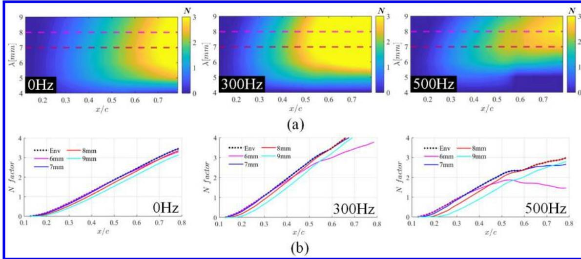
**Fig. 8 (a)  $N$ -factor contours of stationary mode ( $0Hz$ ) and traveling modes ( $300Hz$  and  $500Hz$ ). (b) Envelope  $N$ -factors of stationary mode ( $0Hz$ ) and traveling modes ( $300Hz$  and  $500Hz$ ) along the  $x$  chord.**
