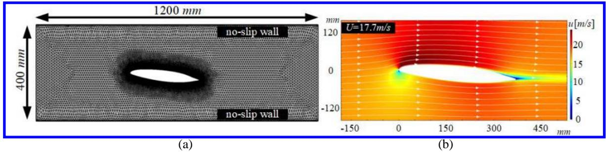
**Fig. 3 (a) The calculation domain and mesh of the CFD simulation. (b) The average velocity field ( $u$ ) with selected streamlines (white arrows).**
