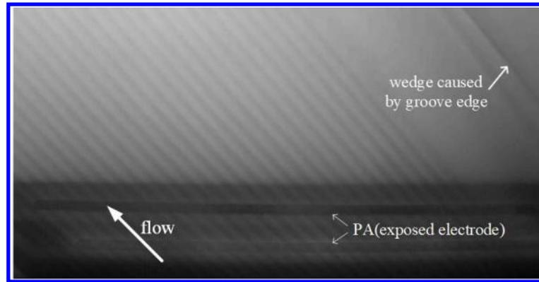
**Fig. 10 IR image of the clean case (DRE with the height of  $200\mu m$ )**
