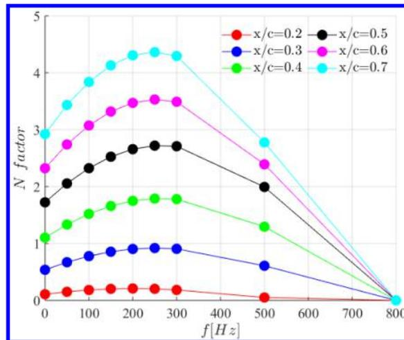
**Fig. 9 Envelope  $N$ -factors of stationary mode ( $0Hz$ ) and traveling modes ( $50Hz$ ,  $100Hz$ ,  $150Hz$ ,  $200Hz$ ,  $250Hz$ ,  $250Hz$ ,  $300Hz$ ,  $500Hz$  and  $800Hz$ ) at various downstream locations**
