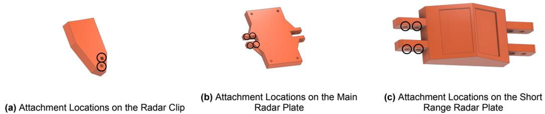
**Figure 12.18:** Attachment Locations of the Radar Plates and Clips
