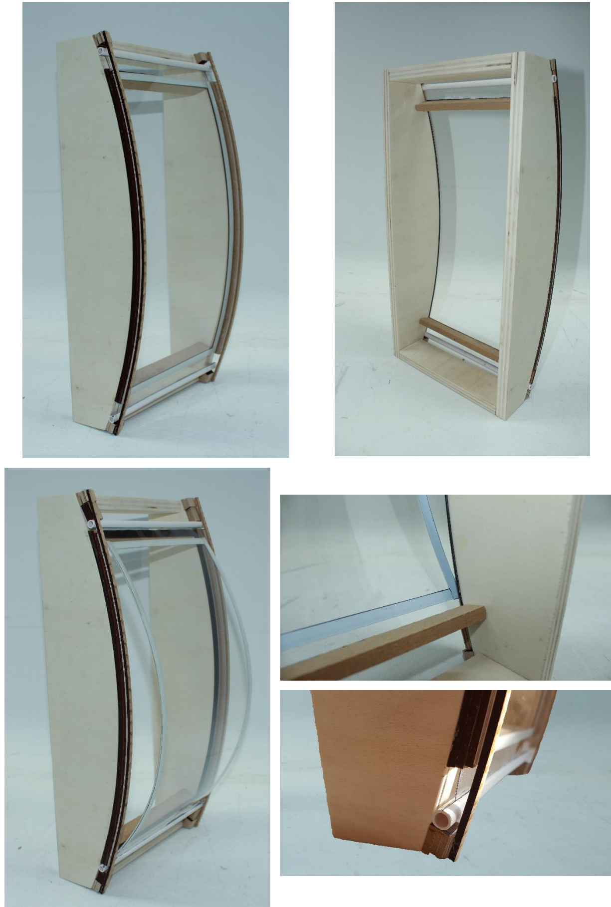
Figure 64 1:5 scale model: top left: isometric view, closed; top right: rear isometric; bottom left: isometric view, open; bottom right: details
