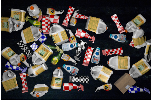
Figure 6.6: Generated image with \pm 50 objects (80% HDPE, 20% Cardboard) using Blender Render completed within 18.43 seconds. Moderate light strength (5) with random textures.
