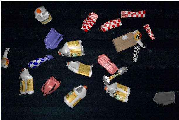
Figure 6.8: Generated image with \pm 20 objects (60% HDPE, 20% Cardboard, 20% PET) using Blender Render completed within 5.99 seconds. Moderate light strength (5) with random textures applied on the objects.
