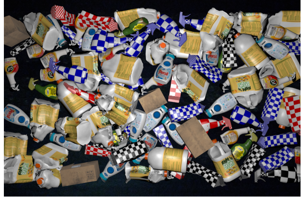
Figure 6.7: Generated image with \pm 100 objects (80% HDPE, 20% Cardboard) using Blender Render completed within 34.12 seconds. Moderate light strength (5) with random textures.
