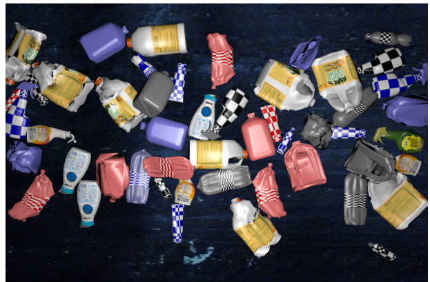
Figure 6.11: Generated image with \pm 50 objects (50% HDPE, 50% PET) using Blender Render completed within 22.94 seconds. Moderate light strength (5) with random textures.
