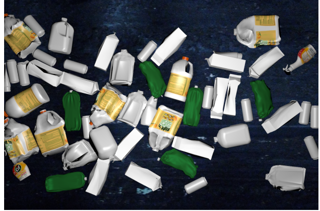
Figure 6.9: Generated image with \pm 50 objects (25% HDPE, 25% Cardboard, 25% PET, 25% Aluminium) using Blender Render completed within 22.42 seconds. Moderate light strength (5) and without random textures.
