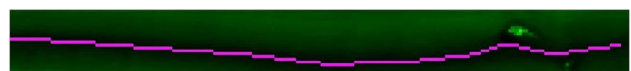
Fig. 4 Minimum of the RT profile representing the fibre for the European ash ( Fraxinus excelsior L.) specimen 263
