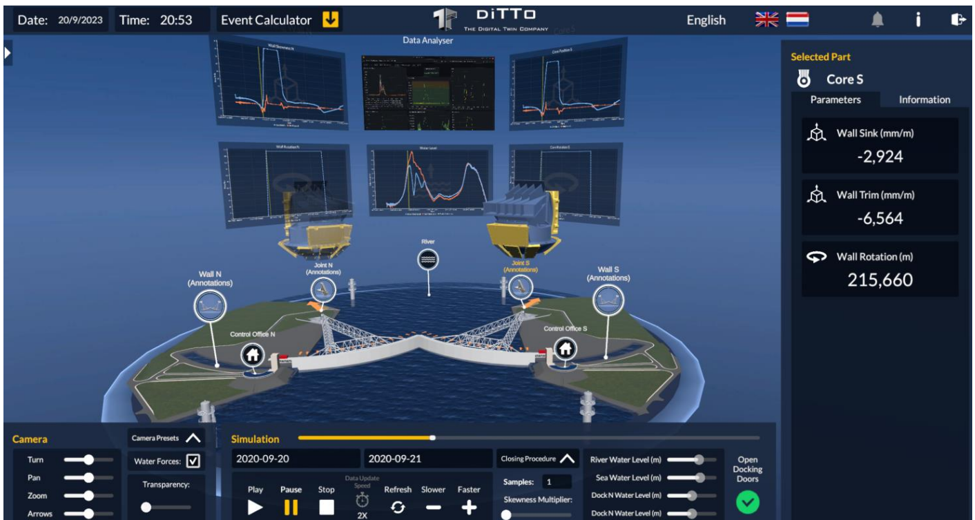
Figure 38: A visualization of the digital twin prototype. It shows the animation of the barrier closing (center), control panels for the simulation or replay of an actual closure (lower panel), clickable panels for data visualization and further data analysis (top panels) and 'live' values of the animated parameters including the option to search for more information (right side)
