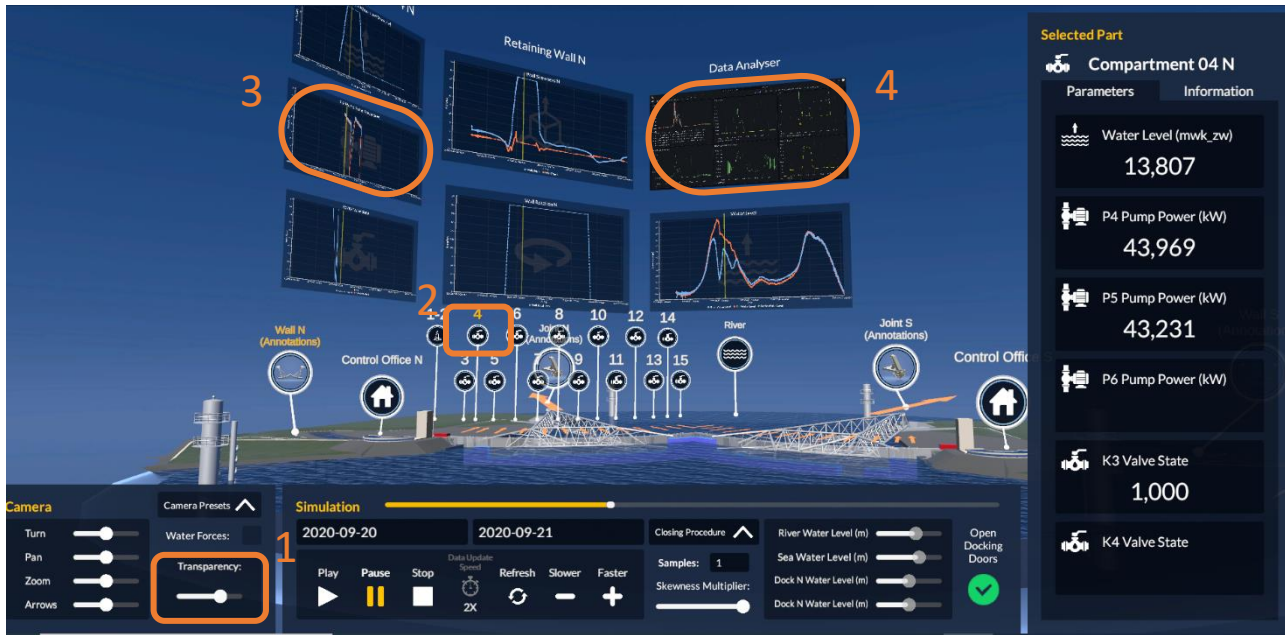
Figure 30: The digital twin is used to 1) visualize the amplified pitch position of the retaining wall, 2) make the wall transparent and notice deviations in compartment 4 in the water levels, 3) open the data of that compartment and 4) further analyse the data. The data in this example is based on measured data during the 2020 test closure.
