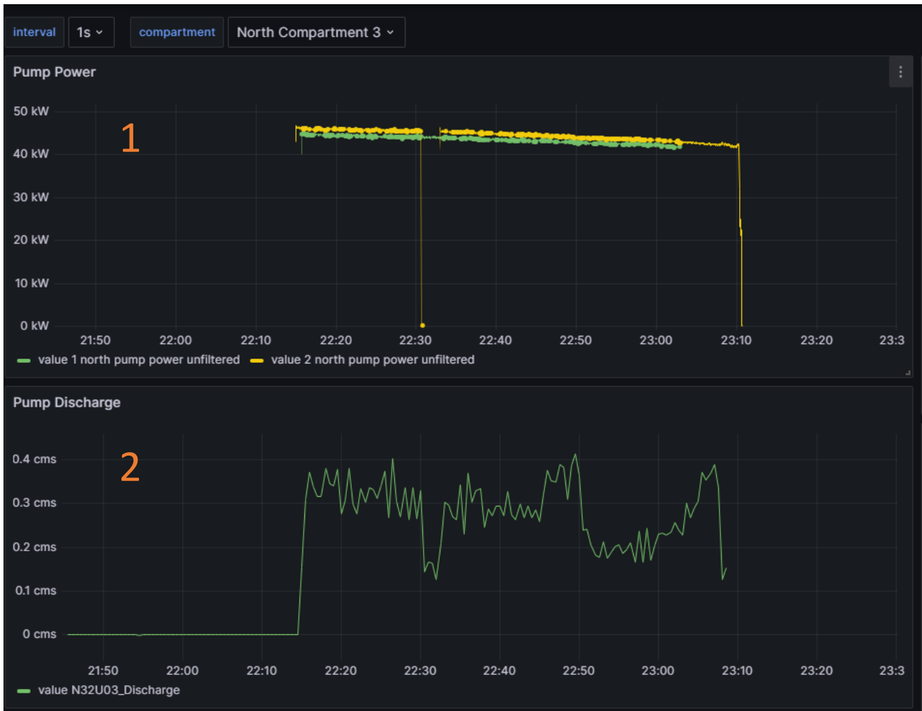
Figure 34: The pump data (1) can be analysed via the data analysis platform in the digital twin, this also provides the possibility to calculate the pump discharge (2).
