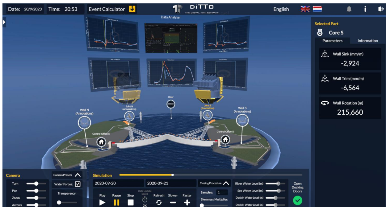
Figure 1: A visualization of the digital twin prototype. It shows the animation of the barrier closing for the actual 2020 test closure (centre), control panels for the simulation or replay of the closure (lower panel), clickable panels for data visualization and further data analysis including water levels, barrier position, pump data and status of valves (top panels) and ‘live’ values of the animated parameters including the option to search for more information (right side)
