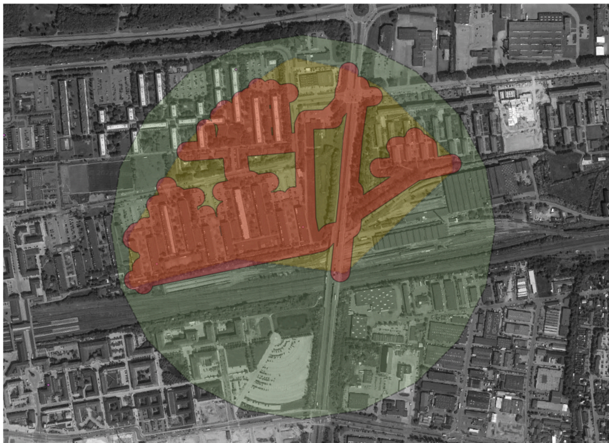
Fig. 2. Types of distance measurement: Types of Distance measurement and accuracy for 500 m in Høje-Taastrup. Red: 25 m Buffered Service Area (BSA), Yellow: Network Distance (ND), Green: Euclidean Distance (ED).
