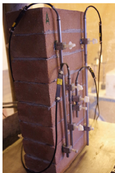
Figure A.5: Compression test on stack-bond prism.
