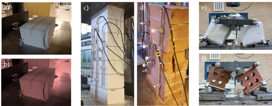
Figure 2.5: Typical failure of CS bricks and clay bricks: (a)–(b) single bricks under compression load; (c)–(d) stack-bond prism in compression; (e)–(f) single bricks under out-of-plane bending loads.
