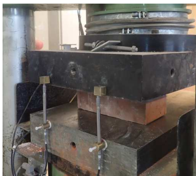
Figure A.4: Compression test on a single brick.
