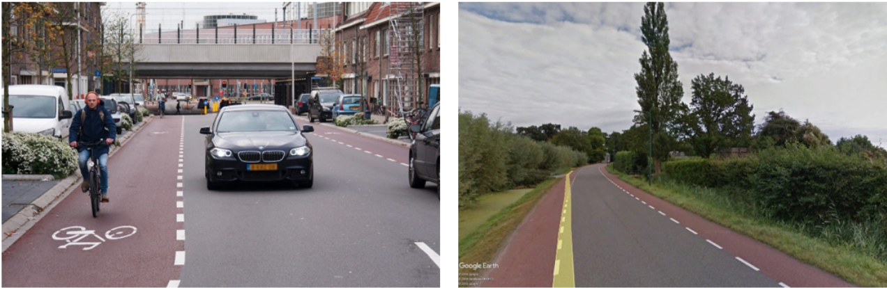
Figure 3.10: Different types of bicycle lanes: an official bicycle lane (a) and a bicycle advisory lane (b)
