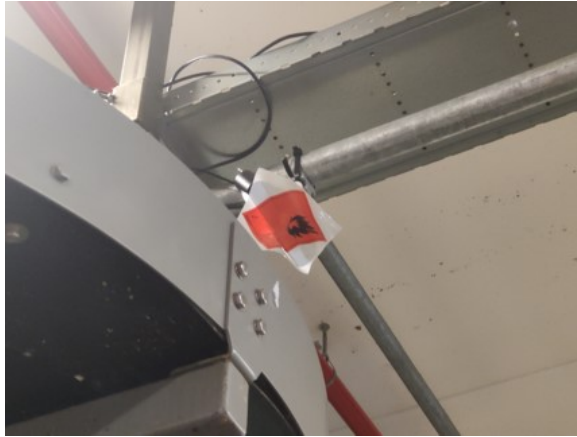
Figure 5.6: A sticker used to block the (stereoscopic) camera overlooking the production line.
