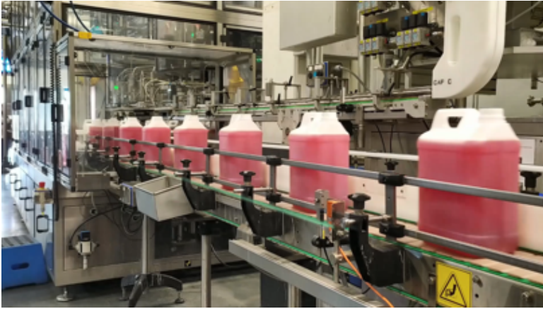
Figure 1.3: Filled detergent canisters exiting the filling and capping machine in an agile factory.
