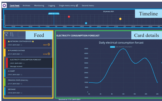
Fig. A1. Hypervision interface of OperatorFabric with feed of cards, selected card details, and timeline.
