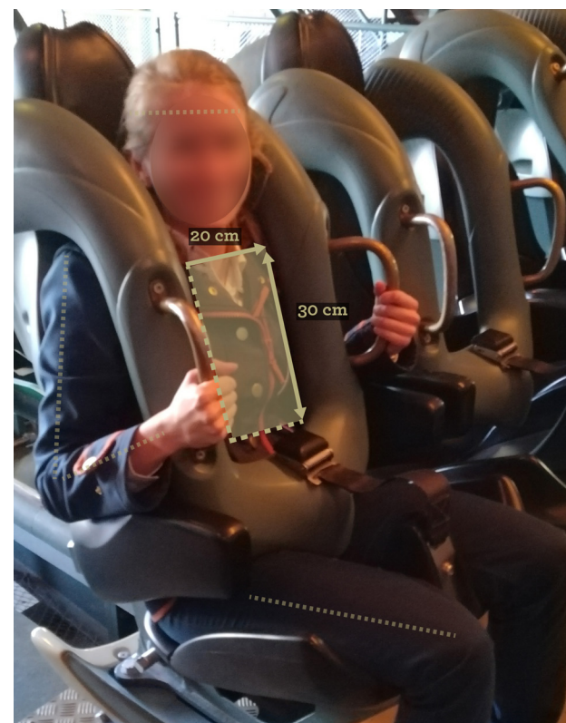
Figure 36. A representation of the workspace that is freely available when the user is sitting in the seat.
