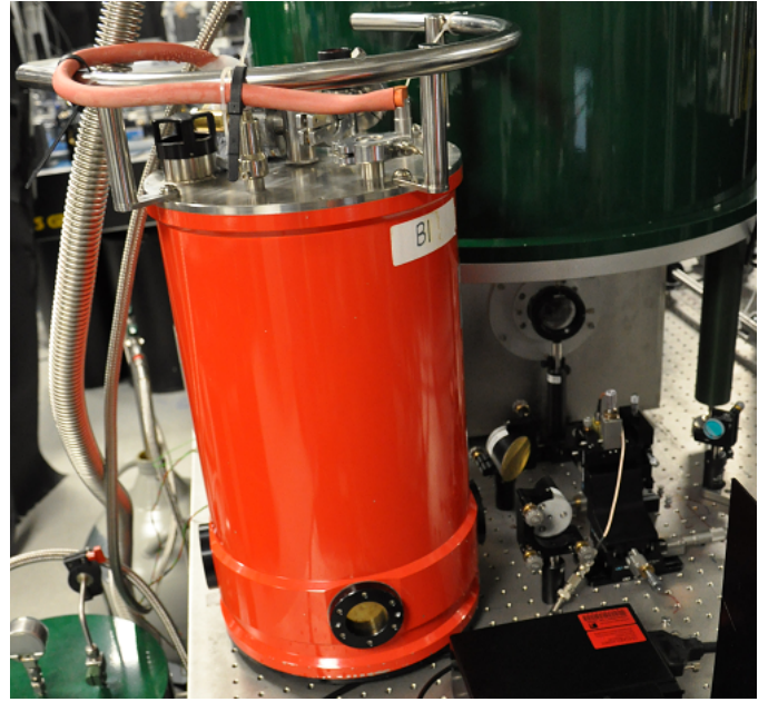
Figure 6. Measurement setup used for the alignment of the photoconductive antenna and the laser beam.
