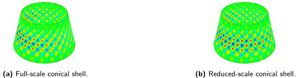
**Figure 6.2:** First eigenmode of the cross-ply composite conical shells, showing radial displacement.
