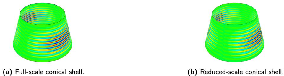
**Figure 5.2:** First eigenmode of the isotropic conical shells, showing radial displacement.
