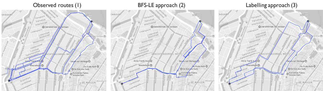
Fig. 5. Routes generated for a given OD pair from the West of Amsterdam to the central train station, for (1) observed routes, (2) BFS-LE approach and (3) Labelling approach.
