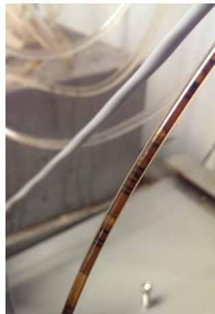
Figure 6.12: Fluids at the outlet of the core; appearing more like an emulsion than a foam.
